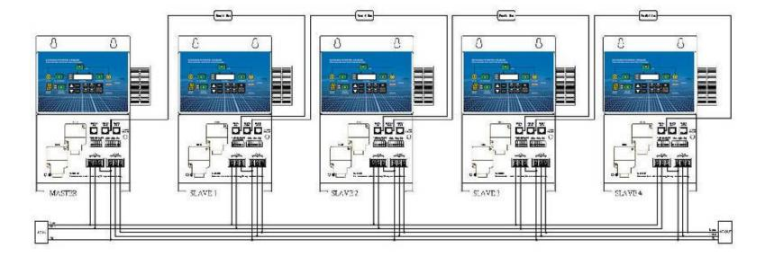
For the MASTER, constant B2-05 and B3-01 must be set. For the SLAVE 1 and 2, constant settings are not required.
